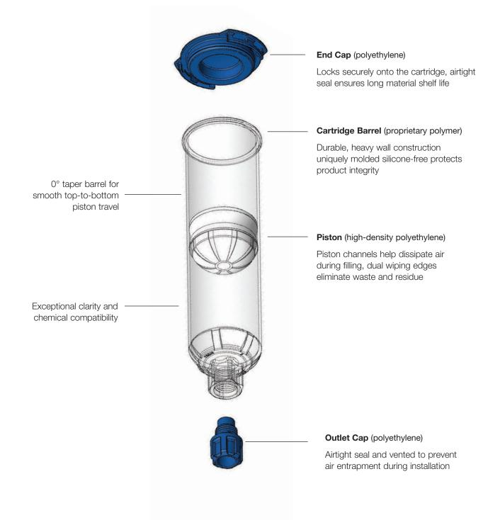
Optimum cartridges are molded from a strong, clear FDA- and RoHS-compliant polymer, with ZeroDraft walls that maintain consistent internal diameters for smooth piston travel.
